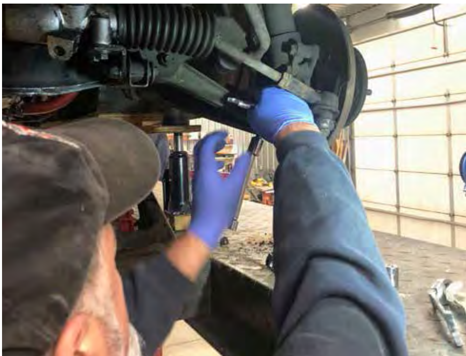
Darren disconnects the LHS radius rods from the lower wishbones and the lower wishbones from the cross-member and pushes them aside
