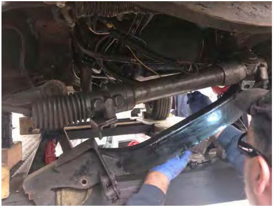
The steering rack is disconnected from the cross-member and allowed to drop slightly while the cross-member is removed. We found that lowering the cross-member on one side provided sufficient room to drop the oil pan
