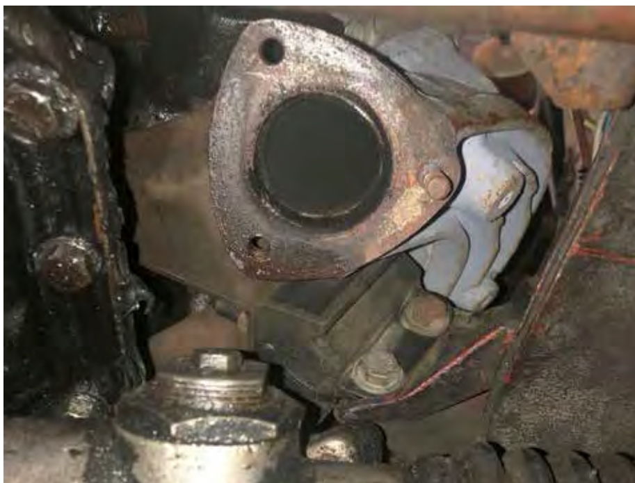
Remove the front section of the LHS exhaust pipe
