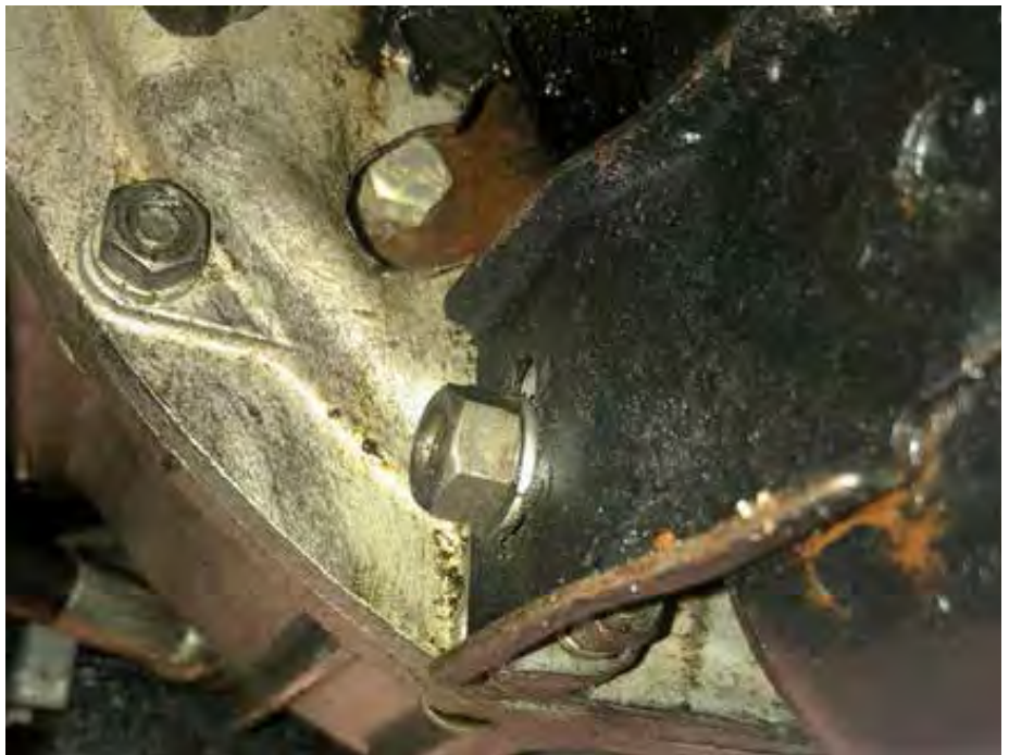
Remove the bolts and two nuts from the oil pan, as well as the bracket on each side attaching it to the front of the rear engine plate. These brackets were not on early Stags nor on 4-speed transmission cars
