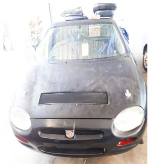
A more substantial task was the venting of the radiator up through the bonnet, this required the modification of spare wheel bay, cutting the bonnet directly above and some ducting to the area. Why did we do this, well the aero on the MGF as standard caused air to go under the car while at the same time a low pressure area develops on the bonnet, which at speeds in excess of 80kph, especially when it is lighted like ours, tends to lift..The venting to the above help to relieve this problem.
