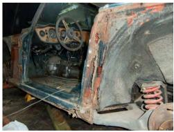
chassis and along with the panels it was taken to Ryan at Shepparton Soda Blasters in Keppell Street for bare metal paint removal. Then back to Mick Doherty's panel works for an undercoat and for John Truman's son Michael to work his magic replacing panels and repairing rust. Mick and his daughter Brook then set about painting all components Mallard Green which is the original colour.
