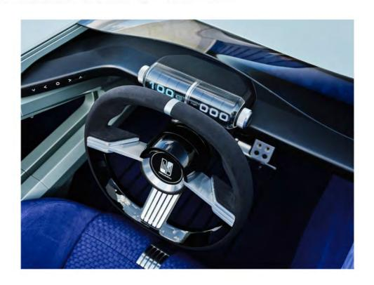
A self-centering dial in the steering wheel displays all vital information while a central binnacle will show road speed, charge levels, and battery range. The spoked steering wheel, which pays tribute to the 'Jabbeke' TR2's wheel in period, will be where the driver can access driving modes, data and the car's navigation system.
